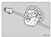
5 Attach the network cable to the 10BASE-T/100BASE-TX port on the machine.
